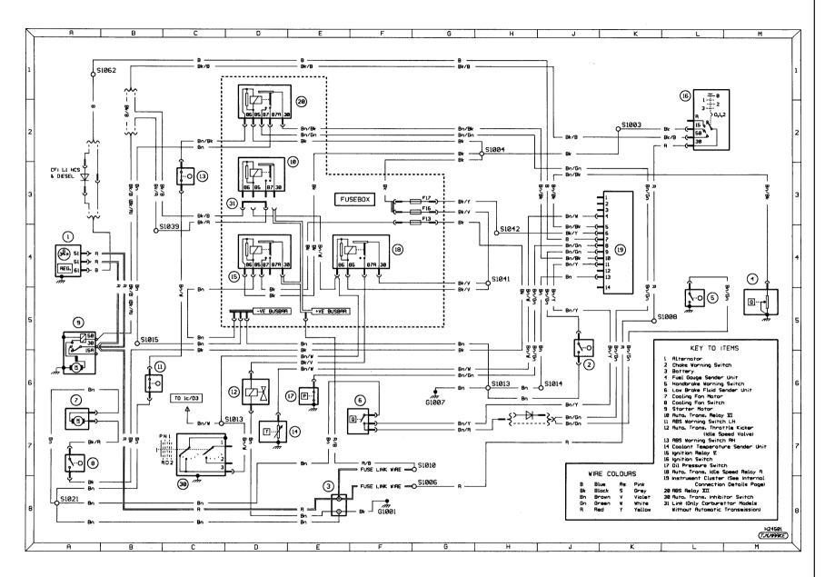
Diagram 1: Starting, charging, cooling fan, ABS, warning lamps and gauges
